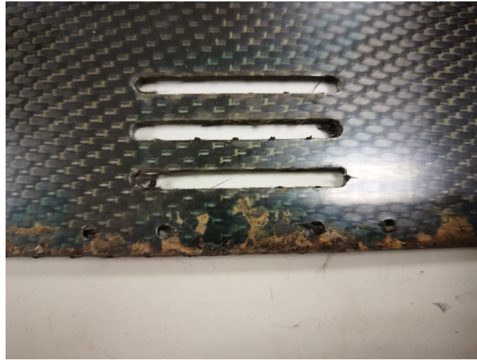
Figure 6.33: Burn marks on edge of front cover
