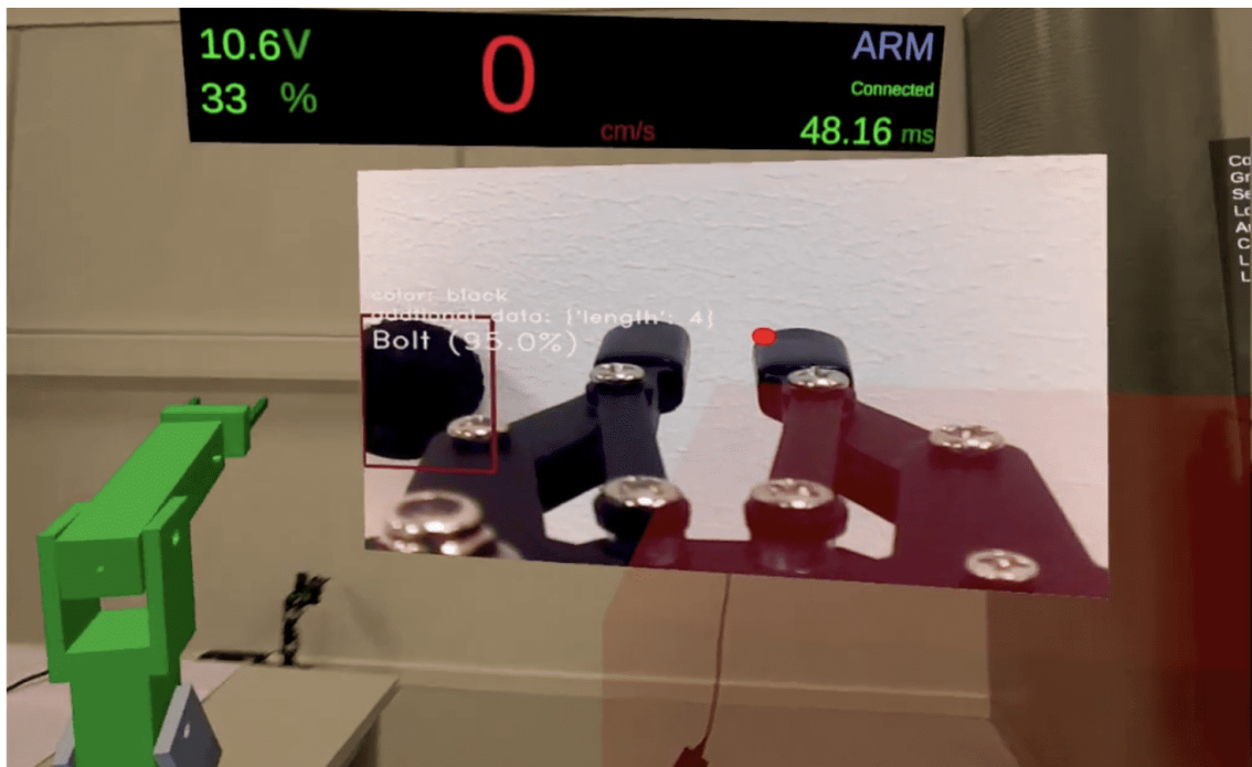
Figure 4.9: Camera monitor in Arm mode (Camera 2) detecting a bolt
