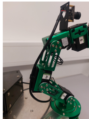
Figure 7.14: This way the cable for the arm camera does not hook itself to the robot.
