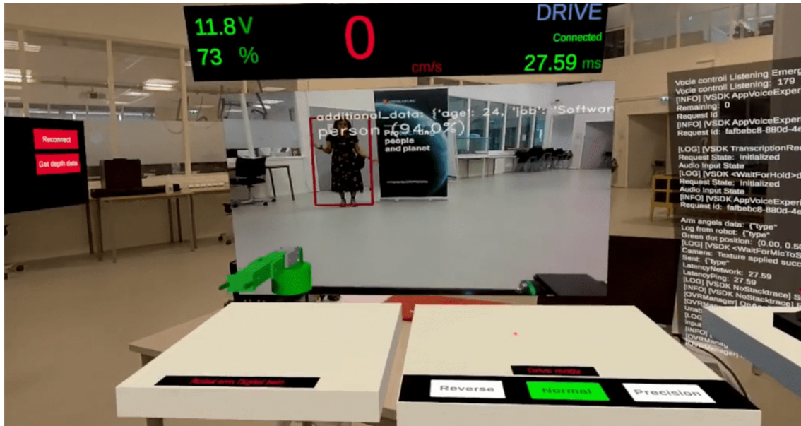
Figure 4.8: Camera monitor in Drive mode (Camera 1) detecting a person
