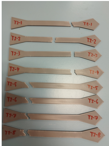
Figure 4.3: The test specimen after the test
